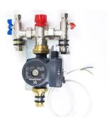
This 1-Group manifold consists of a compact control unit that can be mounted on the wall using a mounting plate. The manifold is suitable for high temperature systems, and is equipped with a thermostat to prevent that too hot water is left in the floor.
