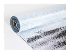
Aluminium reflection foil consists a plastic webbing and an aluminum top layer. The foil reflects heat to the screed and displaces cold through the sub-floor, so it is an extremely effective heat conductor. The foil is designed for direct application under floor heating pipes and can be easily cut to size.
