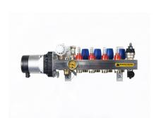
This professional premium MAGNUM control unit is very compact and made of high quality stainless steel type 4301. This allows MAGNUM to give 10 year guarantee on the body of the manifold. The manifold is equipped with a ALPHA2 L pump. Standard with a primary connection above. This pump has a constant pressure, so that it is self-adjusting as there are groups to be closed by a possible after-control (actuator).
