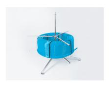
These tubes reel is made of galvanized steel and is equipped with a strong ball bearing. The reel is suitable for almost all standard roll tubes because the uprights of the inner core are manually adjustable. This reel is very robust and has a long life.
